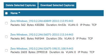
Each packet capture in the list represents a flow of data between devices, and provides information about the devices, ports, and time range to help you narrow down which captures to download.
