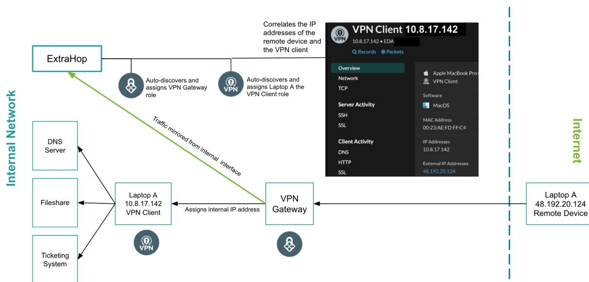
The VPN Client device role is only assigned by the system to devices with an RFC-1918 (or private) IP address. These devices are automatically classified when they are discovered as a child of a VPN Gateway. The VPN Client role cannot be manually assigned.
