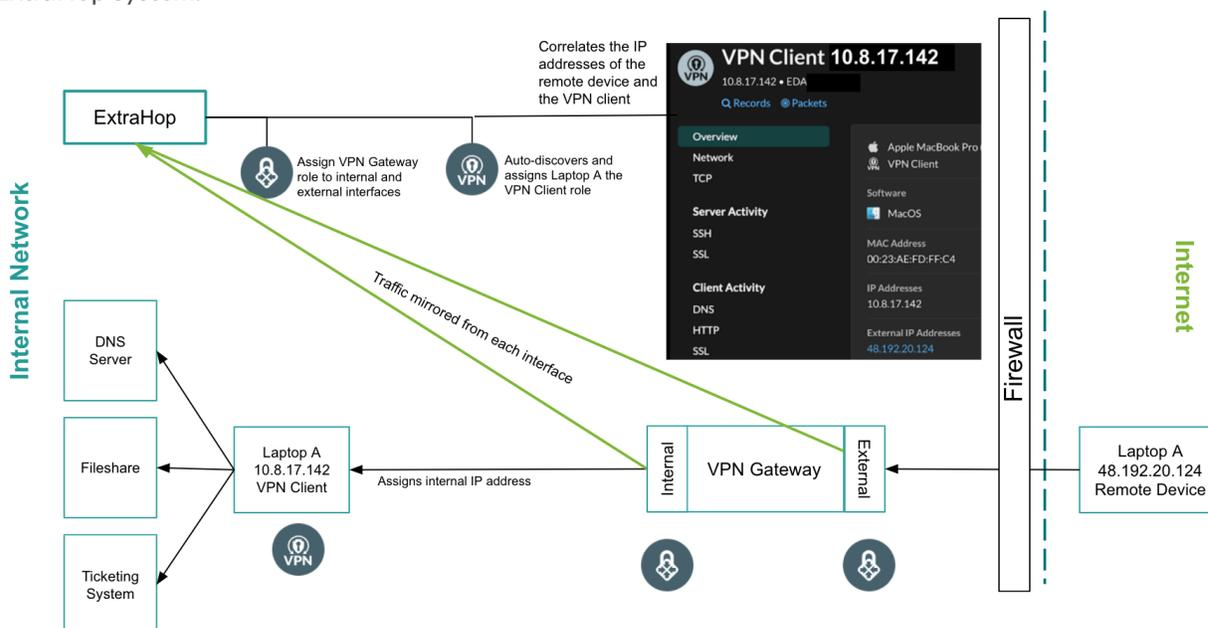
After the VPN gateway roles are assigned to the internal and external interfaces, the ExtraHop system automatically discovers VPN client devices for any RFC-1918 (or private) IP addresses that are assigned through the VPN gateway.
