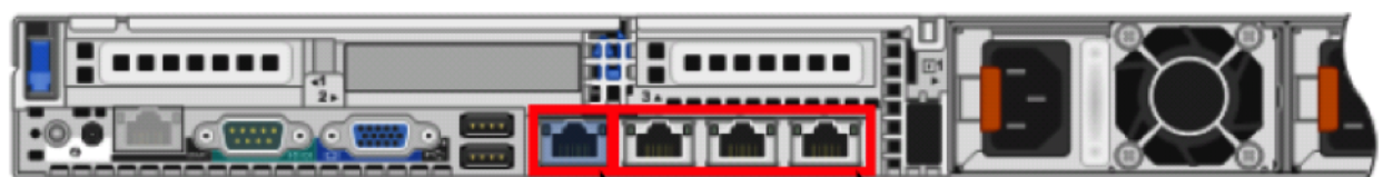
Management Port 1GbE Capture Ports
