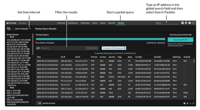
If you change the time interval, the query starts again. Either end of the gray bar displays a timestamp, which is determined by the current time interval. The time on the right displays the starting point of the query and the time on the left displays the endpoint of the query. The blue bar indicates the time range during which the system found packets. You can drag to zoom on a period of time in the blue bar to run a query again for that selected time interval.
