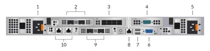
1. Power supply unit (PSU1) to connect the packetstore to an AC power source.
