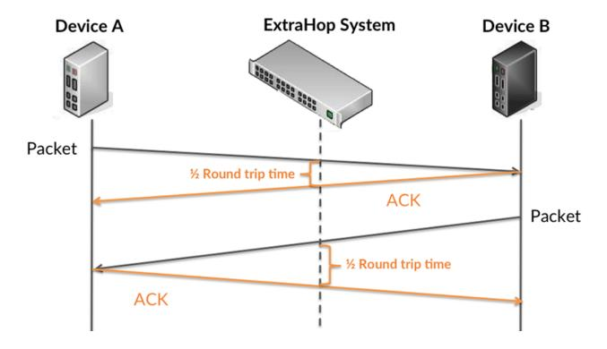
The processing time might be high because the server took a long time to transmit the response (possibly because the response was very large); however, the processing time could also be high because the response took a long time to travel on the network (possibly because of network congestion).
