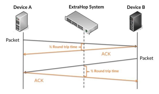
RTT only measures how long an immediate acknowledgment takes to be sent; it does not wait until all packets are delivered. Therefore, RTT is a good indicator of how your network is performing. If you see high processing times, but the TCP RTT is low, the issue is probably at the device-level. However, if the TCP RTT, processing, and transfer times are all high, network latency might be affecting the transfer and processing times, and the issue might be with the network.
