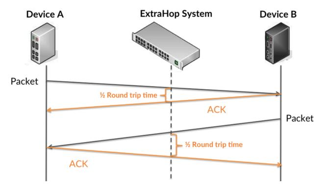
The RTT metric can help identify the source of the problem because it only measures how long an immediate acknowledgment takes to be sent from the client or server; it does not wait until all packets are delivered.
