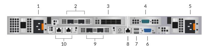
1. Power supply unit (PSU1) to connect the packetstore to an AC power source.
