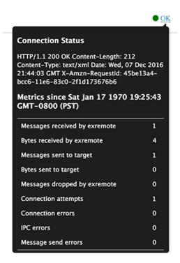
Requests from an ODS trigger to transmit data to the target are asynchronous; there is no support for processing responses to verify the success of a request. The connection details can help you check that the ODS trigger is running and that data is successfully transmitted.
