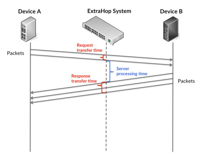
It can be difficult to tell whether an issue is caused by a network or a device from looking only at the processing time, because this metric alone provides an incomplete picture. Therefore the round trip time (RTT) metric is also included in this chart. RTT metrics are a good indicator of how your network is performing. If you see high processing times, but the RTT is low, the issue is probably at
