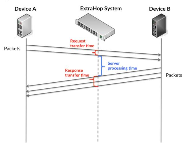
It can be difficult to tell whether an issue is caused by a network or a device from looking only at transfer and processing times, because these metrics alone provide an incomplete picture. Therefore the round trip time (RTT) metric is also included in this chart. RTT metrics are a good indicator of
