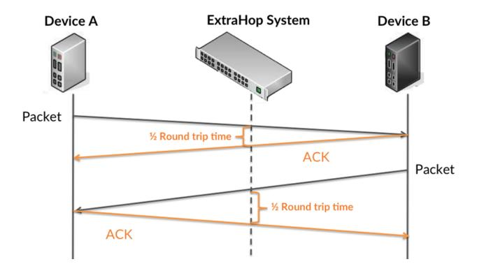
The access time might be high because the server took a long time to transmit the response (possibly because the response was very large); however, the access time could also be high because the response took a long time to travel on the network (possibly because of network congestion).
