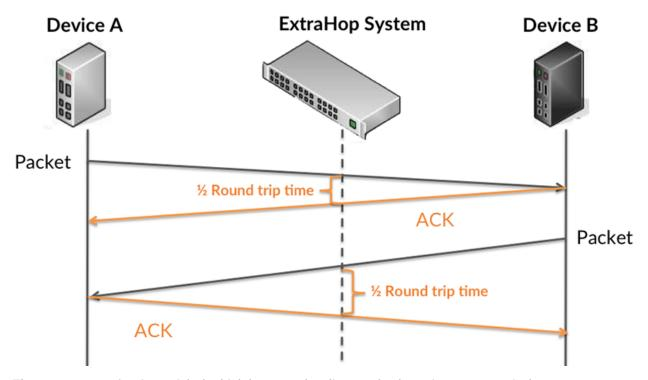
The request transfer time might be high because the client took a long time to transmit the request (possibly because the request was very large); however, the transfer time could also be high because the request took a long time to travel on the network (possibly because of network congestion).
