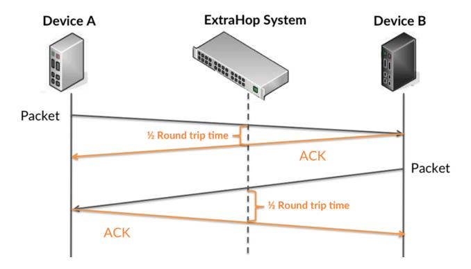
RTT only measures how long an immediate acknowledgment takes to be sent; it does not wait until all packets are delivered. Therefore, RTT is a good indicator of how your network is performing. If the TCP RTT time is high, there might be an issue with the network.
