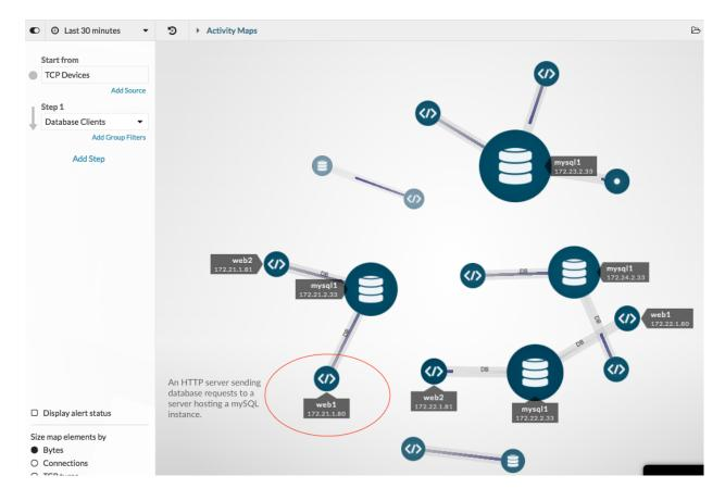
**Tip:** Click the global time selector in the upper left corner to change the time interval and see how database connections have changed over time. You can compare time intervals **Z**, which highlights the newest connections in green.
