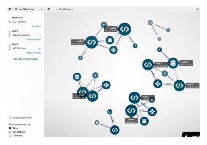
**Tip:** You can learn which of these HTTP clients are part of business-critical applications by applying device group filters. Create a device group I that contains all the devices within an application, and then add a group filter I in Step 2 of the activity map to only see the application devices.
