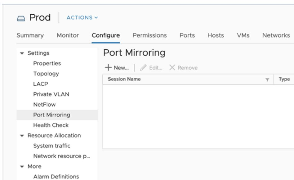
4. Click **New...** to create a port mirroring session to mirror vSphere distributed switch traffic to specific physical switch ports.
