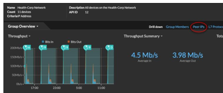
A list of peer devices appears, which are broken down by IP address. You can investigate network bytes and packets information for each peer device, as shown in the following figure.
