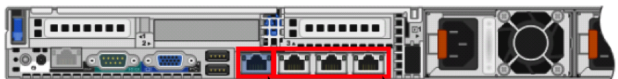
Management Port 1GbE Capture Ports
