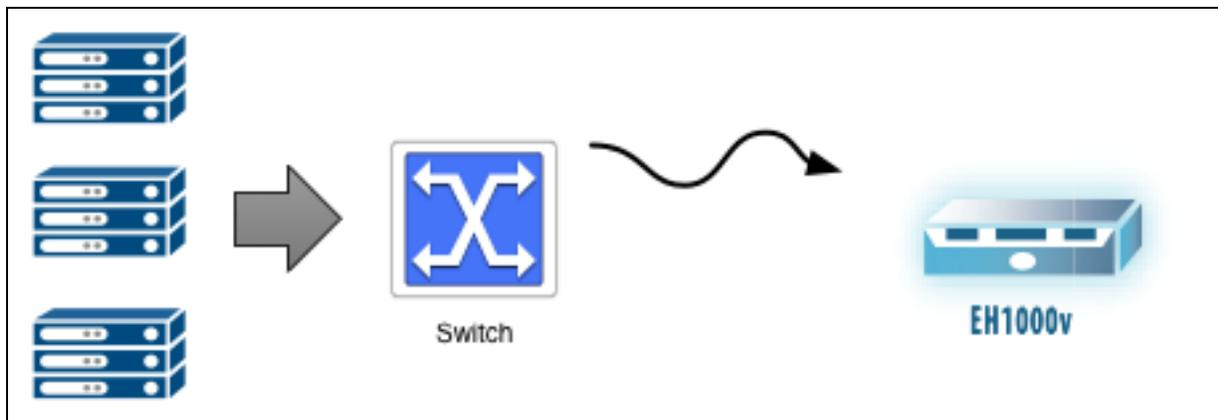
The SPAN port is the name of the port on Cisco switches that mirrors traffic. SPAN stands for Switched Port ANalyzer (SPAN). Different vendors use different names, but spanning has become synonymous for a port on a switch that mirrors traffic. The key thing about a SPAN is that it's all local traffic. You can configure any of the ports on the switch to mirror traffic to an ExtraHop system that has access to the SPAN port.
