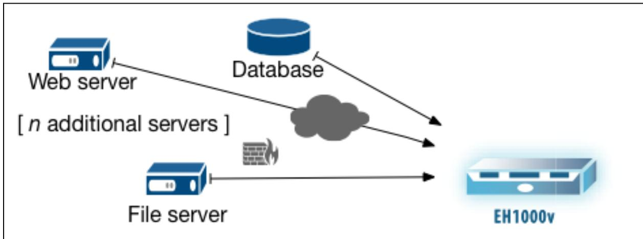
Host-based mirroring requires that you install a software tap on each host you want to monitor. The big advantage of the software tap is that it works with any type of network gear you have. It works independent of the type or version of hypervisor you're running. Host-based mirroring is a way of configuring the adapter on a host to duplicate and forward all traffic to the ExtraHop system. You can install it on Windows or Linux hosts.
