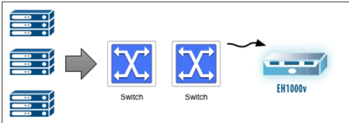
RSPAN is useful if the traffic you're interested in mirroring is more than one switch away from where you can attach your ExtraHop appliance. The "R" in RSPAN stands for remote. You're spanning all the traffic from one switch through any number of additional switches to your target ExtraHop appliance using a dedicated mirroring VLAN. Each switch in the path needs to be configured to carry the dedicated VLAN that contains the mirror traffic.
