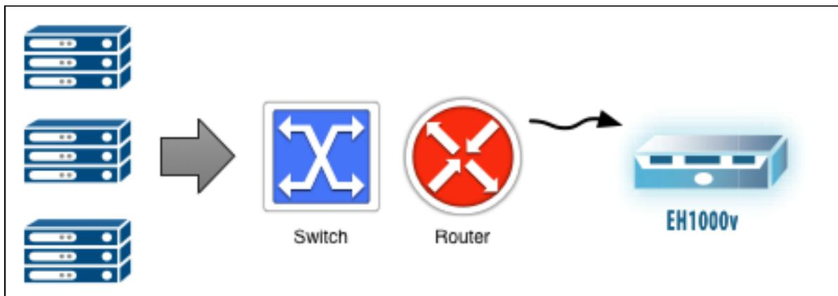
If a Layer 3 (L3) boundary (such as a Router, Firewall, or Layer 3 Switch) sits between the traffic you're interested in mirroring and where you can attach your ExtraHop system, ERSPAN may be helpful to you. To cross the Layer 3 boundary, ERSPAN encapsulates the mirror traffic in a GRE tunnel addressed to the IP address of a capture interface on the ExtraHop appliance. The encapsulated mirror traffic navigates the network just as any other packet would.
